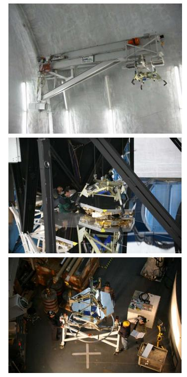
Figure 63: Keck segment-handling system—Enclosure-mounted, segment-handling crane with segment lifting-fixture (top), segment secured on lifting fixture on top of M1 (middle), and segment lowered to handling cart on the observatory floor (bottom).
