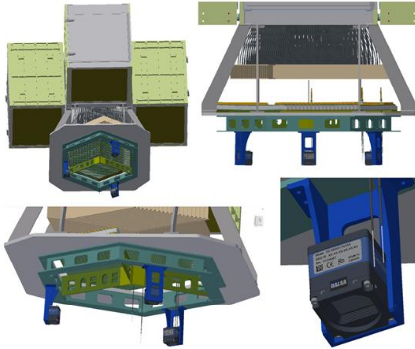
Figure 6. CAD model of three cameras mounted on the Sphinx fiber positioner. Only a few of the positioner spines are shown.
