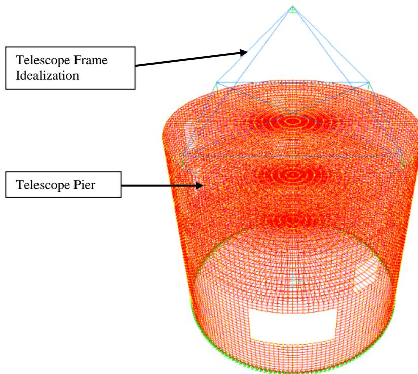
Figure 4: SAP2000 telescope pier and telescope representation finite element model
