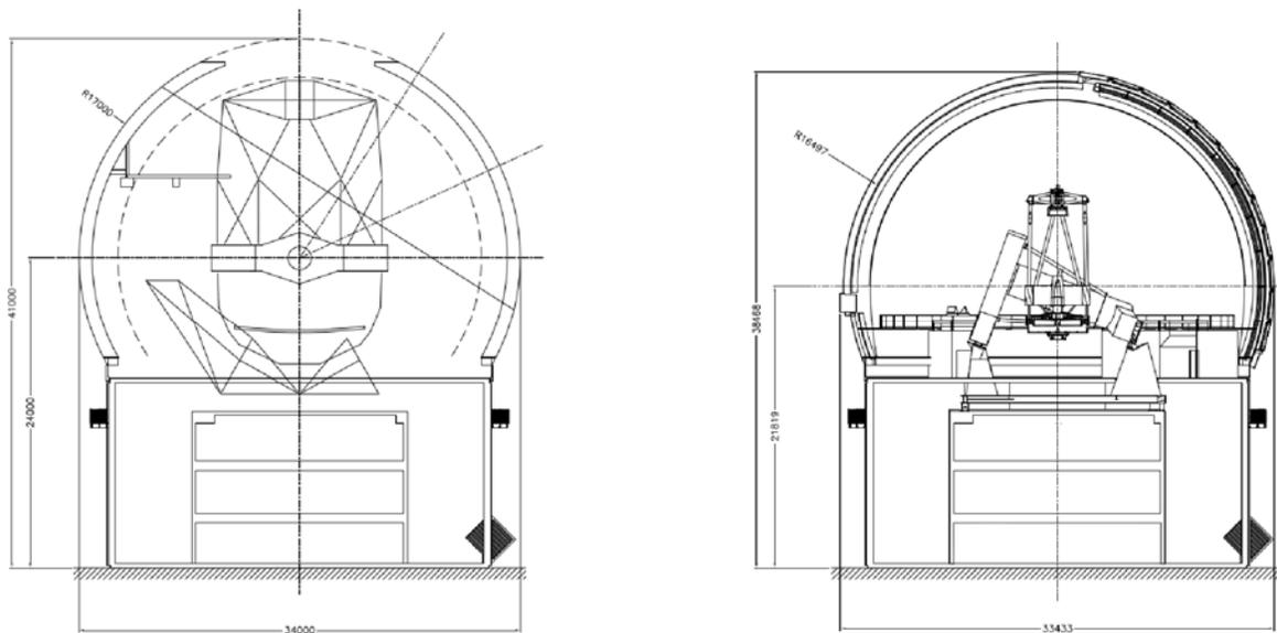
Figure 9: Comparison of the external dimensions of the NGCFHT enclosure (left) and current CFHT enclosure (right).
