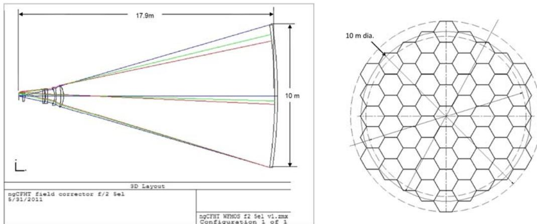
Figure 1: Optical Configuration of NGCFHT – overall focal plane height with wide field corrector (left) and primary mirror with 60 1.44 m segments (right)
