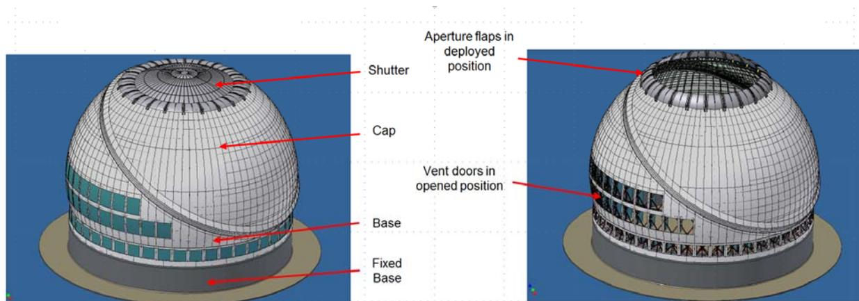
Figure 8: TMT calotte enclosure – vent modules and aperture flips closed (left) and deployed (right).
