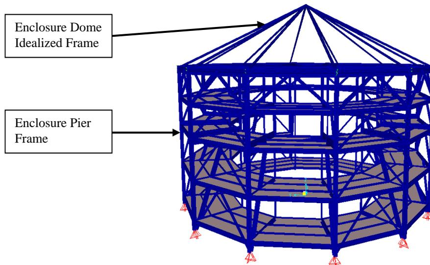
Figure 6: SAP2000 finite element model with the telescope frame idealization
